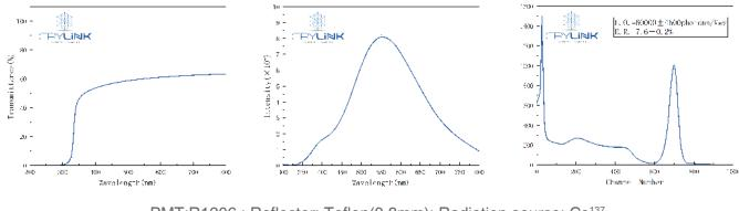
PMT:R1306 ; Reflector: Teflon(0.8mm); Radiation source: Cs<sup>137</sup> HV:650V Light Output :59000 ph/MeV; Energy resolution :7.3%
