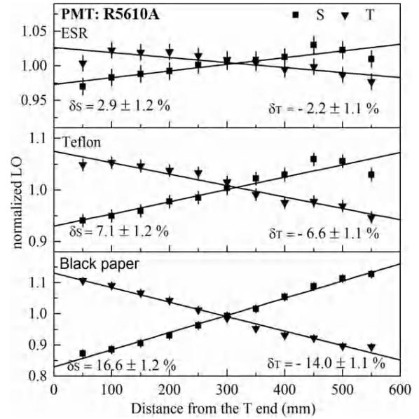
Fig. 7. LRU of the 600-mm-long BGO-SIC-125 crystal wrapped with different reflector materials acquired by Hamamatsu R5610A PMTs. (a) ESR. (b) Teflon. (c) Black paper.
