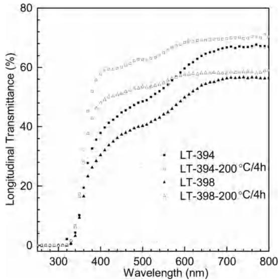
Fig. 6. Optical transmission spectra of the 600-mm-long BGO crystals (SIC-BGO-394 and SIC-BGO-398) along the longitudinal direction before and after air annealing.
