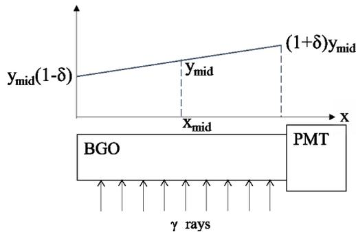
Fig. 3. Schematic of the LRU.
