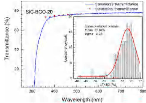
Fig. 4. Optical transmission spectrum of a 600-mm-long BGO crystal along the transversal direction. The theoretical limit of transmittance of BGO is also shown for comparison. Inset: distribution of the optical transmittance at 480 nm along the longitudinal direction of the mass-produced 600-mm-long BGO crystals.
