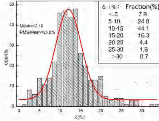
Fig. 5. Distribution of the LRU of the mass-produced 600-mm-long BGO crystals.
