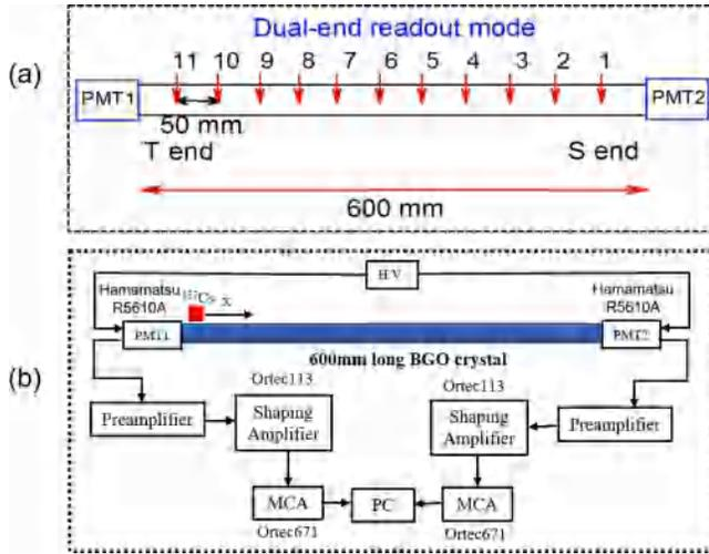
Fig. 2. Schematic of (a) test principle of the LRU and (b) pulse processing chain for the LO acquisition.
