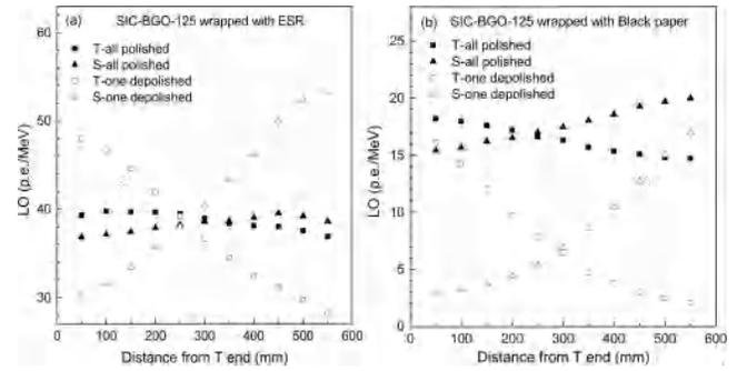
Fig. 8. LRU of the 600-mm-long SIC-BGO-125 crystal wrapped with (a) ESR and (b) black paper.
