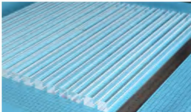
Fig. 1. Mass-produced 25 mm × 25 mm × 600 mm BGO single crystals.
