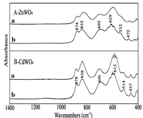
**Fig. 6** FTIR spectra of the as-prepared bulk materials (a) and nanofilms (b)
