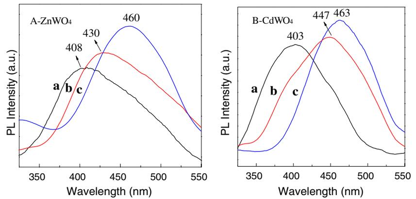
**Fig. 5** PL spectra of the as-prepared nanoparticles and nanofilms: (a)  $\text{ZnWO}_4$  and (b)  $\text{CdWO}_4$
