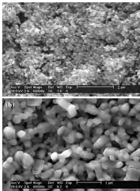
**Fig. 1** SEM images of the as-prepared nanofilms: (a) ZnWO<sub>4</sub> and (b) CdWO<sub>4</sub>
