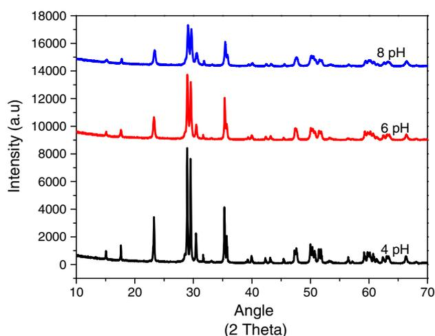
**Fig. 1** XRD patterns of cerium doped  $\text{CdWO}_4$  synthesized at different pH (4, 6, 8)
