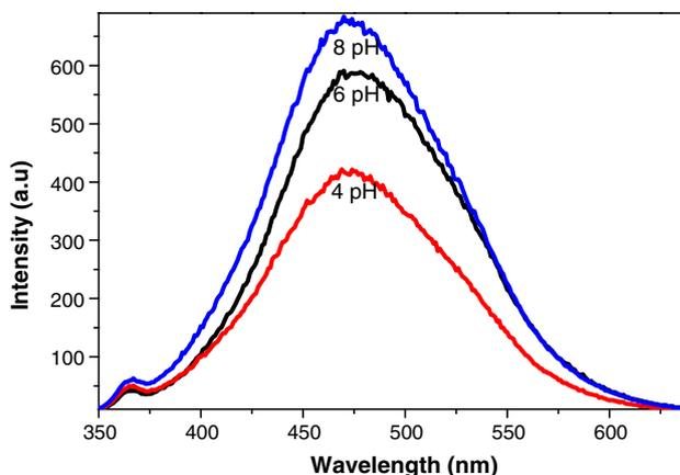
**Fig. 7** PL emission spectra of cerium doped CdWO<sub>4</sub> synthesized at different pH (4, 6, 8) recorded with 270 nm excitation wavelength
