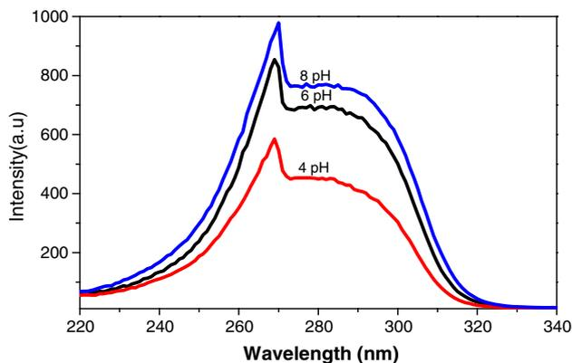
**Fig. 6** Excitation spectra of cerium doped CdWO<sub>4</sub> synthesized at different pH (4, 6, 8) recorded with 475 nm emission wavelength
