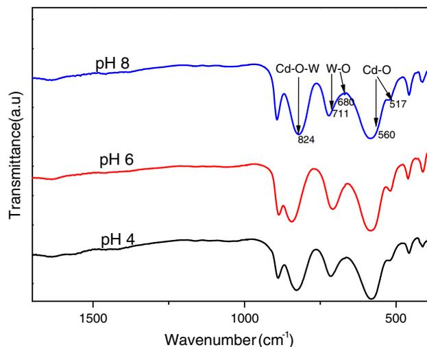
**Fig. 3** Room temperature FTIR spectra of cerium doped CdWO<sub>4</sub> synthesized at different pH (4, 6, 8)
