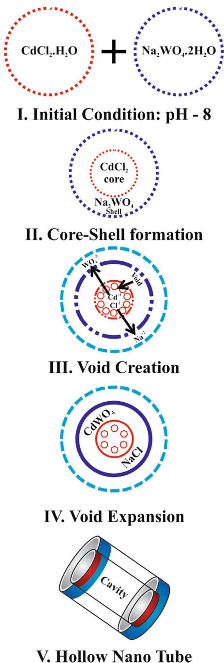
**Fig. 5** Approach A for formation of hollow nano tube
