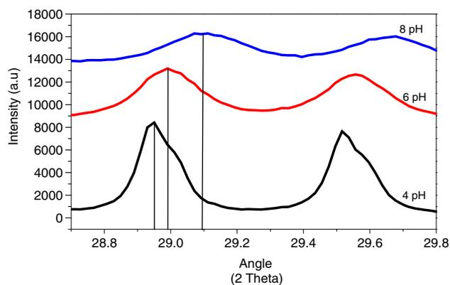
**Fig. 2** Shift of reflection peak of cerium doped CdWO<sub>4</sub> synthesized at different pH (4, 6, 8)
