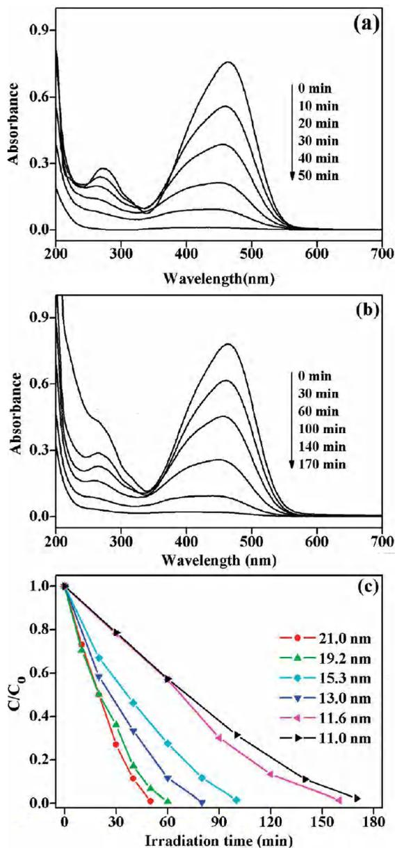
**Figure 8.** Time-dependent absorption spectra of MO solution in the presence of (a) 21 nm CdWO<sub>4</sub> and (b) 11 nm CdWO<sub>4</sub> under UV light irradiation; (c) photocatalytic activities of CdWO<sub>4</sub> nanostructures at different particle sizes.
