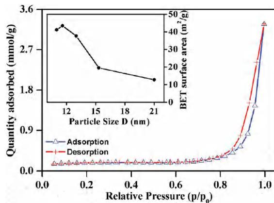
**Figure 5.** Representative nitrogen desorption/adsorption isotherms for 21 nm CdWO<sub>4</sub>. Inset illustrates the relationship between specific surface area and particle size of CdWO<sub>4</sub> nanoparticles.
