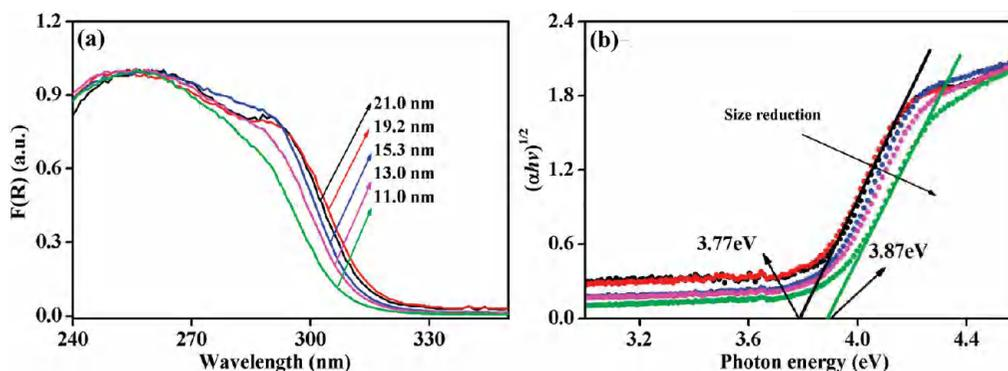
**Figure 6.** (a) UV–visible diffuse reflectance spectra and (b) energy dependence of  $(\alpha hv)^{1/2}$  for  $\text{CdWO}_4$  nanocrystals at different particle sizes.
