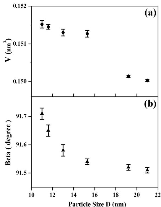
**Figure 3.** Particle size dependences of (a) lattice volume,  $V$ , and (b)  $\beta$  angle of CdWO<sub>4</sub> nanocrystals.
