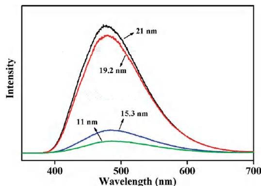
**Figure 7.** Photoluminescence spectra of  $\text{CdWO}_4$  nanocrystals at given particle sizes under the measurement conditions: solid-state samples, 290 nm excitation, and room temperature.
