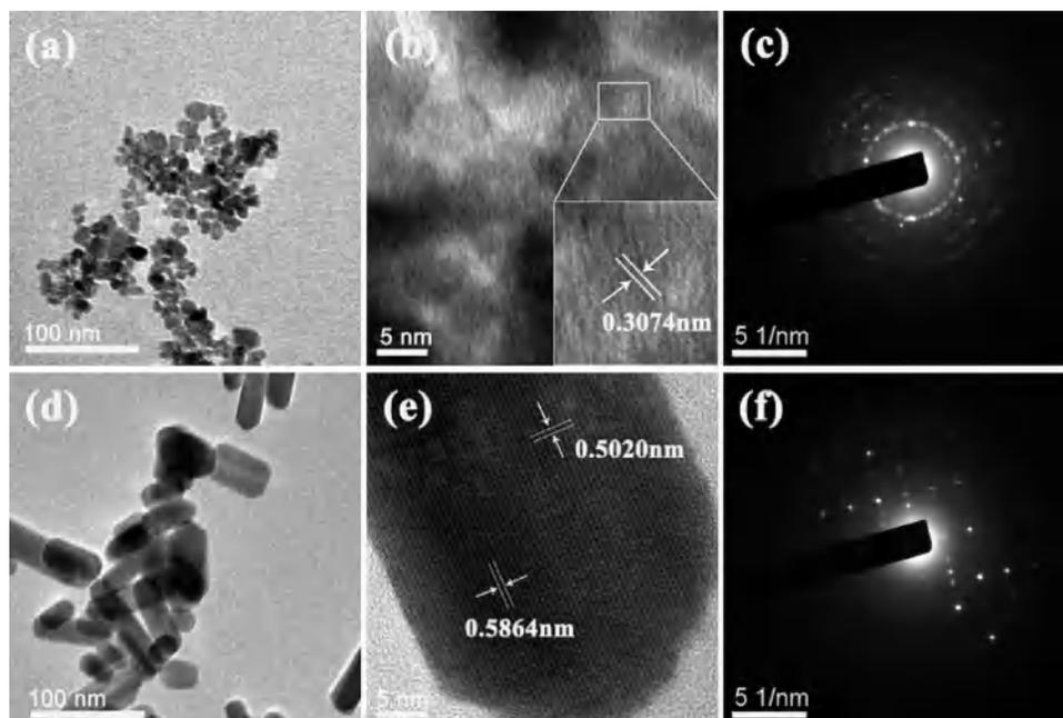
**Figure 2.** (a) TEM, (b) HRTEM, and (c) SAED images of 11 nm CdWO<sub>4</sub>; (d) TEM, (e) HRTEM, and (f) SAED images of 21 nm CdWO<sub>4</sub>.
