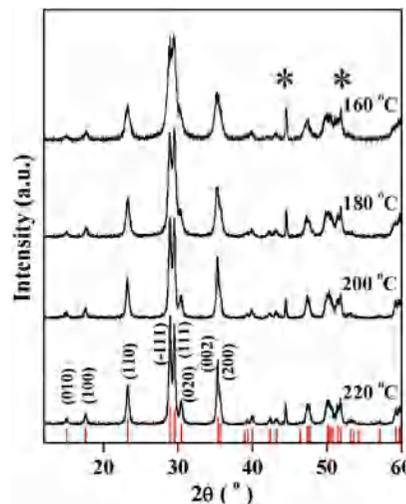
**Figure 1.** Selected XRD patterns of CdWO<sub>4</sub> prepared at different temperatures. Vertical bars represent the standard diffraction data for bulk CdWO<sub>4</sub>. Bracketed numbers are the Miller indices for specific crystal faces. Symbol \* represents the diffraction lines of internal standard nickel.
